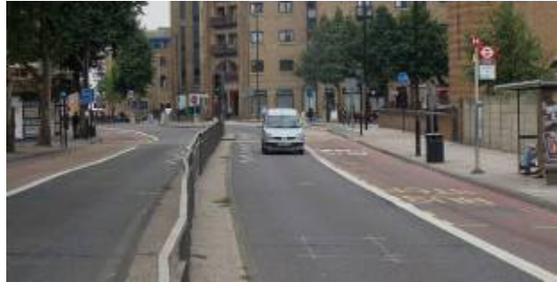
Central railings; increases speed & takes space
